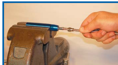
STEP 2 Flare braid using a twisting motion.
