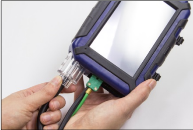
Fig. 44: Pulling the condensate trap out of the analyzer
