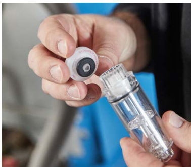
Fig. 48: Filter holder with water stop filter.
