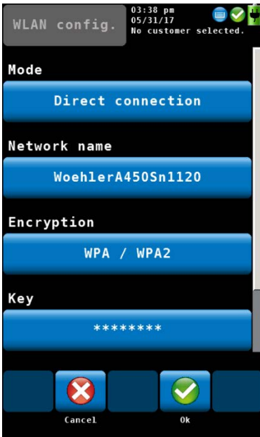
Fig. 35: WLAN configuration – Direct connection
