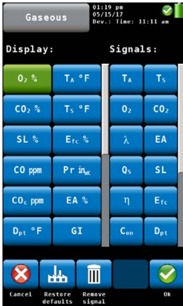
Fig. 38: Configuration of the readings segment.
