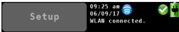
Fig. 37: „WLAN connected“ appears in the upper display, alternating with the selected customer
