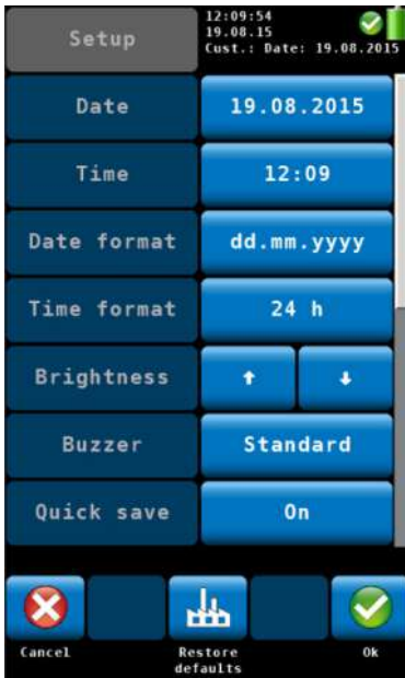
Fig. 57: Setup menu, the scroll bar shows that there are more parameters available.
