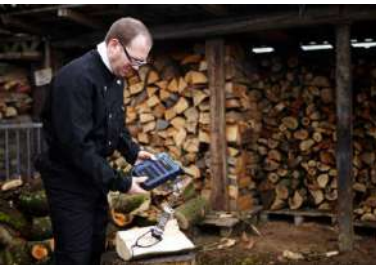
Fig. 40: Wood moisture measurement with Probe Wöhler HBF 420.
