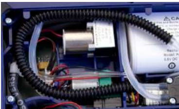
Fig. 75: Corrugated tube, correctly positioned
