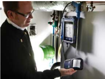
Fig. 33: Printing the readings of the Wöhler A 550 on the Thermoprinter Wöhler TD 100.
