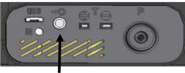
Fig. 39: Connectors for the wood moisture probe at the bottom of the analyzer
