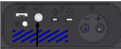
Fig. 44: Connectors for the wood moisture probe at the bottom of the analyzer
