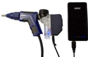
Fig. 59: Probe grip with Peltier Cooler and USB power bank
