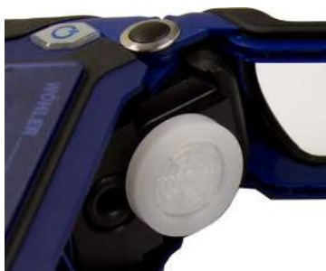
Fig. 69: Water stop filter
