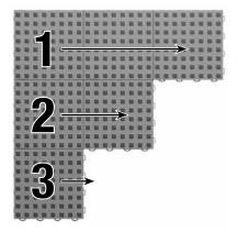
Tiles should be arranged so that tabs are on the left and top, while loops are on the right and bottom. Install the tiles by following the pattern on the diagram. For the best results, work from left to right completing an entire row at a time.
