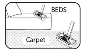
Apply light consistent pressure and slowly pass it along the surface (1" per second) to insure the area being treated has a chance to come to full temperature killing pests and their eggs.
