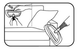
The clothes / fabric tool with the cotton cover is ideal for treating bedding, furniture, pillows, and carpet areas around bed posts and base boards. Start by installing the supplied cotton cover on the clothes – fabric / smooth surface tool. Apply light consistent pressure and slowly pass it along the surface (1" per second) to insure the area being treated has a chance to come to full temperature killing pests and their eggs.
