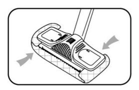
The floor cleaning head with micro fiber cover is also great for treating large surface areas such as bedding, furniture, and carpet areas. Start by installing the supplied micro fiber cover on the floor cleaning head. The micro fiber cover thermal core maintains full temperature during use and allows the floor cleaning head to glide over fabric or carpet.
