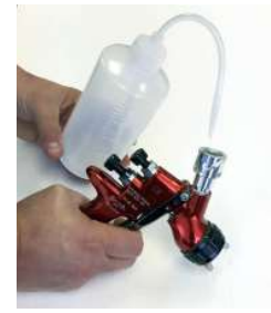
Pre clean Fluid Passageway
