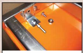
2. Drill 5/16" (8mm) holes at four marked locations. Attach MAIN FRAME to top of chest with SHORT CARRIAGE BOLTS (a) and NUTS (d). Tighten NUTS inside tool chest.
