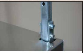
5. Place UPRIGHTS (C) into MAIN FRAME BRACKETS with top SHELF SUPPORTS pointing toward front of tool chest. Attach UPRIGHTS with LONG HEX BOLTS (b) and FLANGE NUTS (d). Finger tighten nuts.
