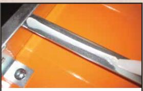
3. Apply a 1/8" bead of pure silicone from a calking gun onto top surfaces of MAIN FRAME. Dab some silicone around carriage bolt heads to ease disassembly if needed.
