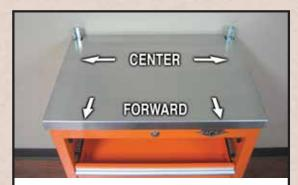
4. Set COUNTERTOP onto MAIN FRAME. Press down to COMPLETELY FLATTEN silicone. Slide COUNTERTOP FULLY FORWARD with equal overhang on sides. Use masking tape to hold COUNTERTOP while silicone dries.
