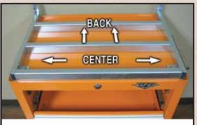
1. Place MAIN FRAME (A) on tool chest in the CENTER and against BACK lip. Mark the location of four square mounting holes on top of tool chest. Remove MAIN FRAME.
