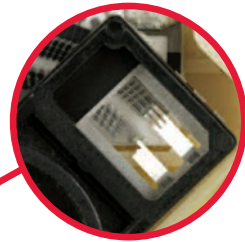
Damaged Worn, broken contacts cause inaccurate readings.
