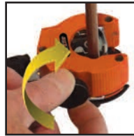
Spring-loaded automatic cutter. Snug down onto tubing, then turn knob 360°.
