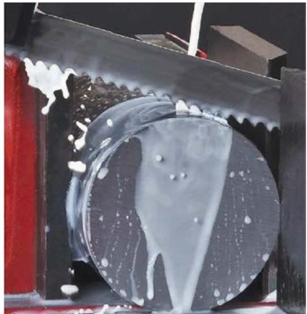
Start to cut material at reduced cutting rate
