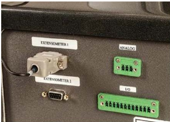
Digital I/O is available on all MMx and FMx test frames. Analog I/O is only available using the MMS or MMD test frames.
