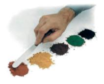
ASTM designation C-979 standard specification for pigments for integrally colored concrete limits the amount of pigments to no more than 10% of the total weight of the cementitious material in the mix.
