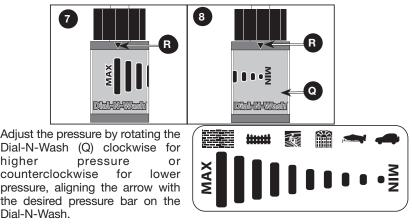
**NOTE:** To apply chemicals the black low pressure nozzle must be installed and the Dial-N-Wash must be in the MAX pressure setting.
