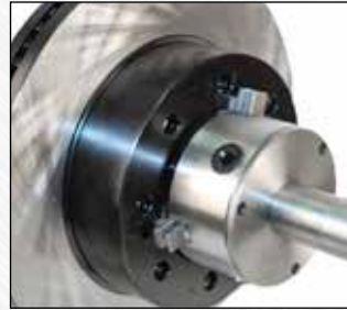
Quick-Chuck with Truck Jaws Mounted Rotor
