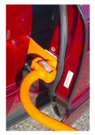
Move the door towards the door jam and rest the Alignment Bar on the door catch (You can use the center opening or either notch on the Alignment Bar).
