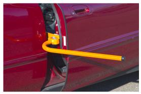
Gently move the handle up or down to adjust the door to the desired position.
