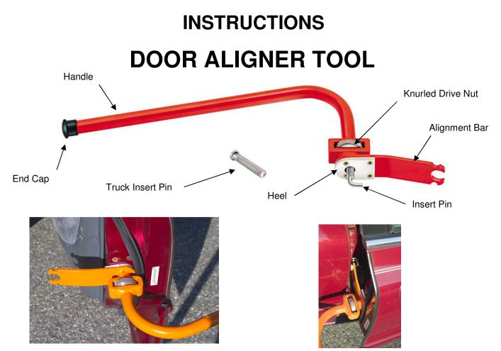
Open vehicle door. Slide Insert Pin into the open door latch until it completely locks.
