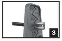
Insert the stripped wire into the terminal. Completely close the jaws to crimp the terminal. Squeeze the handles together to form the first crimp.
