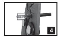
Insert the insulated portion of the wire into the appropriate cavity and squeeze the handles to form the tabs around the insulation.
