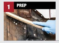
Remove loose scale with a wire brush. Clean with **SEM Solve** to remove oil, grease and dirt. Blow off with compressed air.
