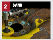
Remove loose rust scale by sanding, grinding or using a wire brush.
