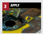
Apply 2 medium coats of **Rust Trap** with a brush or spray gun. First coat should not achieve full coverage and second coat should be applied in the same manner while first coat is still wet. Allow final coat to cure for 8-24 hours before returning part to service.
