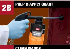
Clean surface with SEM Solve or XXX Universal **Surface Cleaner** where applicable. Shake bottle of **Rust Preventer** for 1 minute. Spray 1 - 2 coats at 35 - 45 psi.
