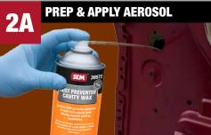
Clean surface with SEM Solve or XXX Universal Surface Cleaner where applicable. Remove cap from **Rust Preventer**, attach straw or **Rust Preventer Aero Wand.** Apply 1 - 2 coats.
