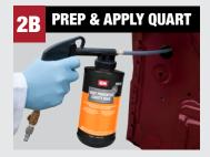
Clean surface with **SEM Solve** or **XXX Universal Surface Cleaner** where applicable. Shake bottle of **Rust Preventer Cavity Wax** for 1 minute. Spray 1-2 coats at 35-45 psi.
