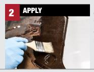
Dip smaller parts or brush onto larger parts. When applying **Rust Mort** by brush, keep product wet throughout the conversion process.
