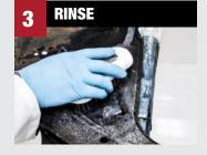
After conversion or removal, rinse treated areas using a brush with clean water to remove any **Rust Mort** that isn't dry. Dry thoroughly to avoid flash rusting. Proceed with body filler if needed, then topcoat.
