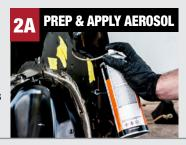
Clean surface with SEM Solve or XXX Universal Surface Cleaner where applicable. Remove cap from Rust Preventer Cavity Wax, attach straw or Rust Preventer Aero Wand. Apply 1-2 coats.
