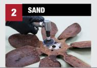
Remove loose paint and rust scale by sanding, grinding, or using a wire brush. Removing additional rust will result in a better final appearance. Sand painted areas with P220 grit. Blow off surface and clean again with SEM Solve or XXX Universal Surface Cleaner.
