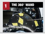
Rust Preventer Cavity Wax is easily applied with a 360° spray pattern when using the Premium Undercoat Applicator & Wand or the Rust Preventer Aero Wand.
