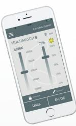
With the new BLUETOOTH lighting control app you are able to control and adjust both the light output and the colour temperatures, along with a range of other useful, wireless functions improving daily work efficiency.
