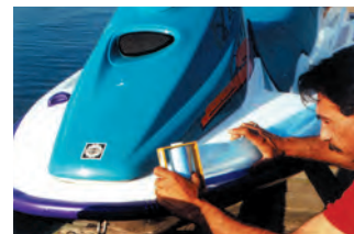
21" for masking along edge of jet ski between hull top and bottom
