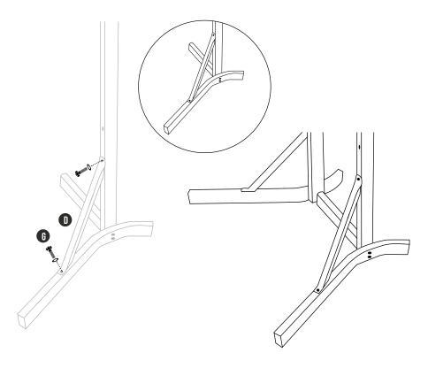
3. Screw the base feet (Part B) into the designated spots on the base legs (Part A)
