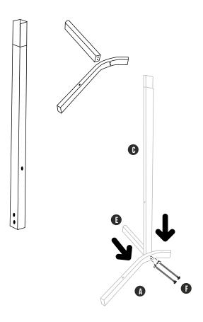
2. Attach the angular support braces (Part D) using the 1/2" bolts and washers (Part G) as shown.
