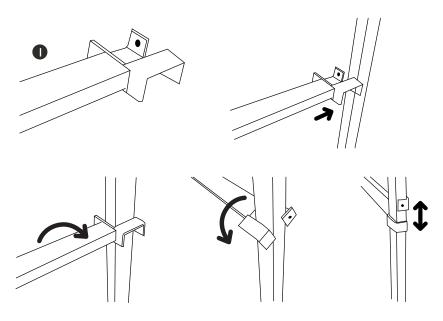
**6.** Tighten the locking knobs on the end so that the mounting arms are secure.
