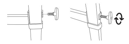
NOTE: Mounting arms may be positioned at varying heights to accommodate the frame of your specific bicycle.
