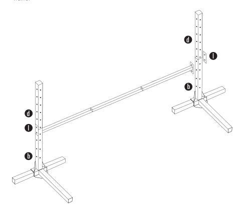
**6.** Use two (2) 3 ½" hex bolts (m), with two (2) washers and a lock nut on each, to attach the rack arms (I) to the frame. Attach the first arm to the lowest two holes possible, and the second arm in the highest two holes possible. Repeat on the other side. (You may find it helpful during this part of the process to use one wrench to hold the bolt in place and use a second wrench to turn the lock nut).
