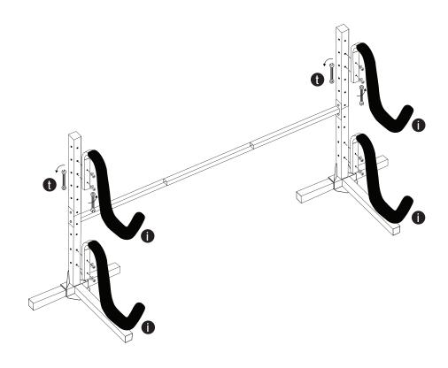
7. The kayak rack should be fully assembled. If possible, drill a bolt down into the floor with the anchor brackets (r) to stabilize the unit in a permanent position, preventing it from tipping over. If not, make sure that the weight is always evenly distributed, and if only storing one kayak, store it on the lower rack.
