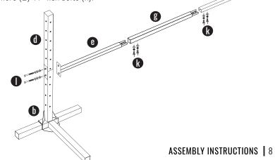
**5.** Attach the assembled cross bar from step 4 to the second assembled base from steps 1-3, using the second cross bar plate (I), and two (2) of the 2 ¾" hex bolts (I), with two (2) washer and a lock nut on each bolt to attach the plate to the frame.
