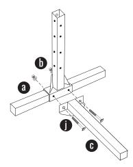
2. Attach the leveling feet (s) by placing two (2) hex nuts (that come with each leveling foot) and an anchor bracket (r) on each one. Make sure the anchor bracket has one nut on both sides of it. Lean the assembled base to one side and attach the leveling feet (s) to the welded nuts on the underside of the base (a) and base leg (c). Repeat this process on the second assembled base.
