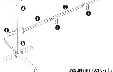
**5.** Attach the assembled cross bar from step 4 to the second assembled base from steps 1-3, using the second plate (I), and two (2) of the 2 ¾" hex bolts (I), with two (2) washer and a lock nut on each bolt to attach the plate to the frame.
