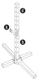
**4.** Place the plate (I) on one side of the post (d) and the base post (b) and place the cross bar end (male) (e) on the opposite side. Use two (2) 2 ¾ " hex bolts (I) to attach the plate (I) and the cross bar end (male) (e) to the holes where the post and base post connect. Then, connect the central cross bar (g) to the cross bar end (male) using two (2) ¾ " hex bolts (k). Finally, connect the cross bar end (female) (f) to the central cross bar using two (2) more 3/4" hex bolts (k).
