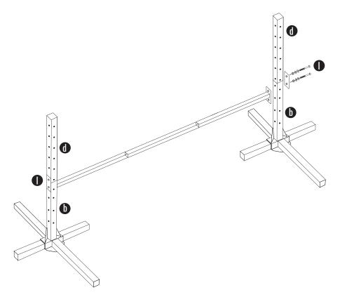
**6.** Attach the first two (2) arms (i) to the lowest two (2) holes possible on opposite sides of the assembled base. Use two (2) 4 1/2" hex bolts (m) to secure the two (2) arms (i) in place. Then, place and secure the next two (2) arms (i) on the highest holes on the assembled base. Repeat on the other assembled base. (You may find it helpful during this part of the process to use one wrench to hold the bolt in place and use a second wrench to turn the lock nut).
