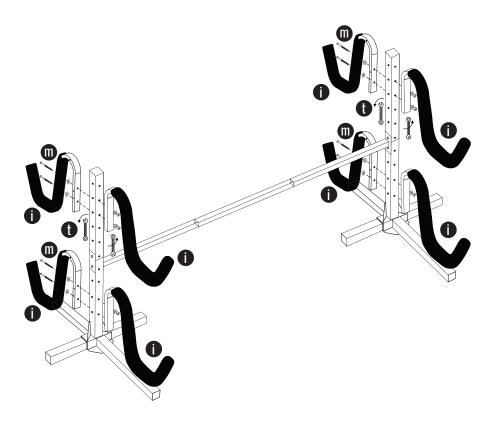
7. The kayak rack should be fully assembled. If possible, drill a bolt down into the floor with the anchor brackets (r) to stabilize the unit in a permanent position, preventing it from tipping over. If not, make sure that the weight is always evenly distributed, and if only storing one kayak, store it on the lower rack.
