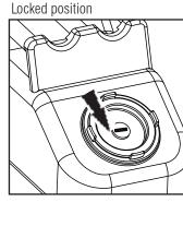
Opening and closing front door and top lid. Pull up on lid while turning the latch. Be careful not to let the lid fall freely as it could cause damage to the tool box.
