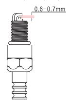
Standard Spark Plug: E6TC/E6RTC/BPR6HS
