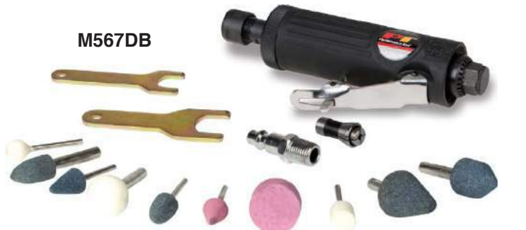
M567DB Die Grinder, (5) 1/4" shank mounted stones, (5) 1/8" shank mounted stones, 1/4" and 1/8" collets, 2 collet wrenches, storage case
