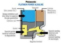
Alkaline Plus Power AA and AAA batteries utilize new zinc alloy, electrolytes, and special organic inhibitors which dramatically reduces gas build up generated within the cell. Panasonic has also developed a unique gasket material which has increased resistance to degradation. This new material and the highly specialized sealing method, when combined with new zinc alloy, electrolytes and organic inhibitors, dramatically reduces the possibility of electrolyte leakage.
