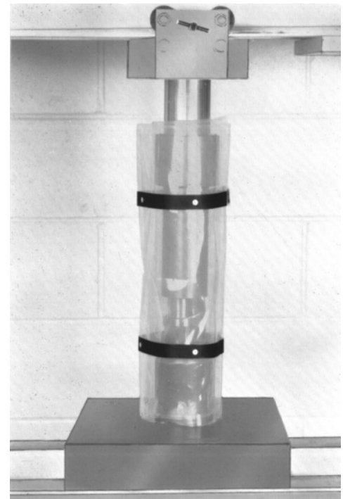
Blanket covers housing, bearing being installed, and installing tool.
