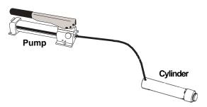
IMPORTANT: Some spring return cylinders, or rams, have a cavity in the rod which forms an air pocket. This type of cylinder or ram should be bled when positioned upside down or lying on its side with the port facing upward.
