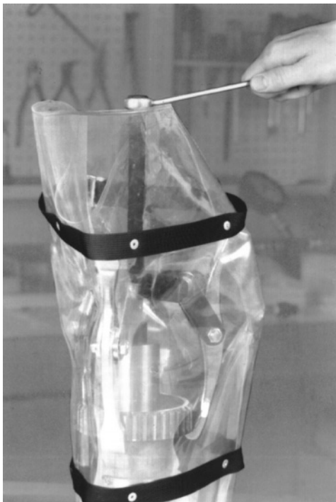
Blanket covers both the part being pulled and the puller.
