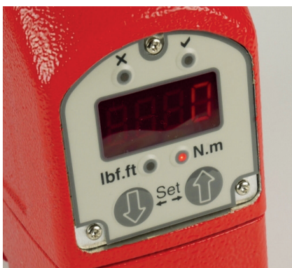
Internal Control (IC) Panel
