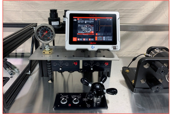
T-Box™ 2 at the center of a test bench for hydraulic torque wrenches
