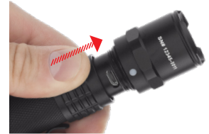
Sliding collar hides USB port when not in use
