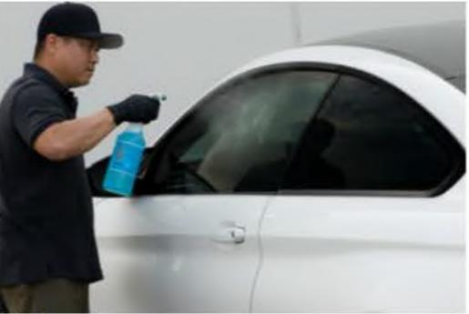
Step 1: Spray sufficient amount of lubricant on the glass surface.
