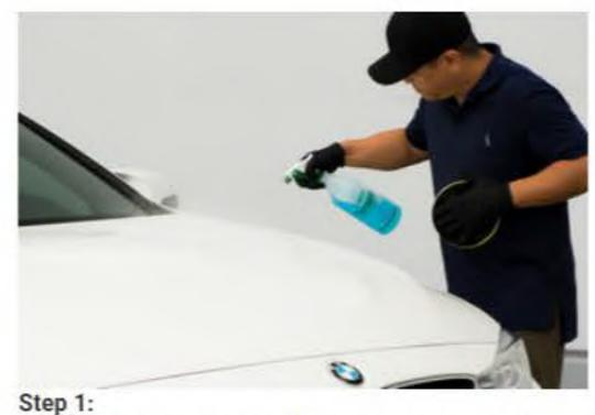
Spray sufficient amount of lubricant on the paint surface.
