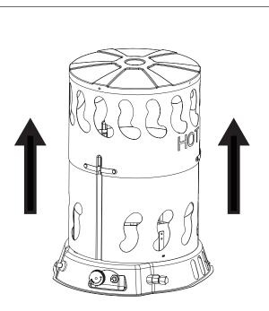
STEP 2: LIFT OUTER SHELL STRAIGHT UP. CARE MUST BE TAKEN TO PROTECT HANDS DURING LIFT.
