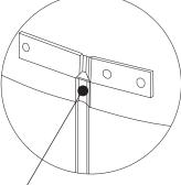
Make sure clip goes into slot in lower shell. 3 Places STEP 3: LIFT OUTER SHELL UNTIL ALL THREE CLIPS ENGAGE SLOTS IN LOWER SHELL. WHEN THIS HAPPENS, THE SCREW HOLES WILL LINE UP. Lock shells together and
