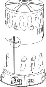
STEP 4: LOCK THE CLIP INTO PLACE WITH 3 SCREWS AS SHOWN. THE HEATER MUST NOT BE OPERATED UNLESS THE OUTER SHELL IS PROPERLY EXTENDED AND FULLY LOCKED INTO PLACE.
