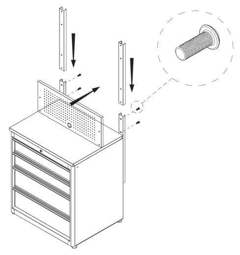
Slide two A posts onto the B posts. Make sure to leave enough room at the top for the wall cabinet.
