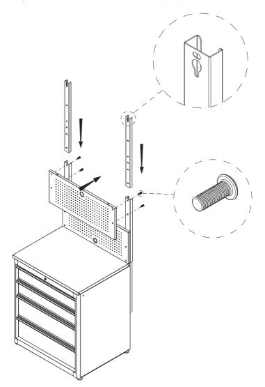
Insert two M6 x 16 hex socket head screws into the top holes of the wall cabinet, but do not fully tighten. Hang the wall cabinet on the top of the posts, then fully tighten the screws.
