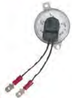
035760-10 Conversion Capsule Converts fuel level reading from standard direct site gauge to electric dash-mounted gauge (33-240 ohms).
