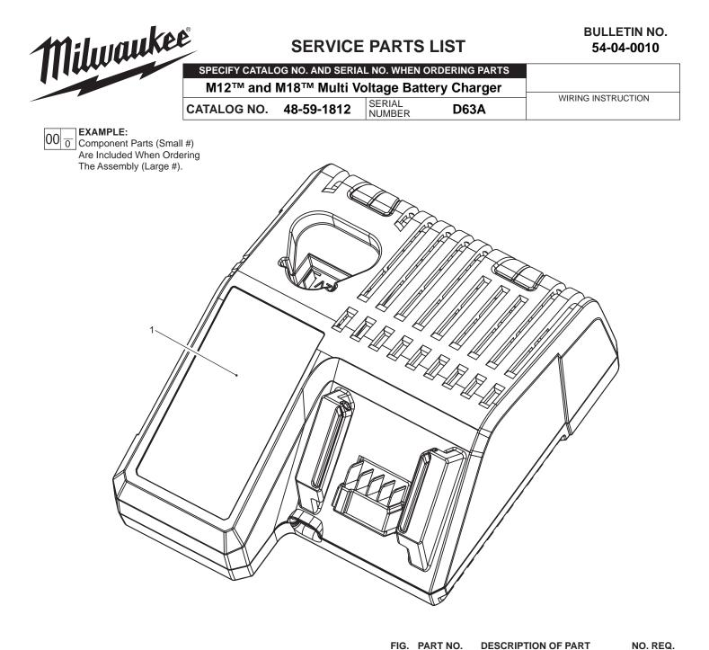
FIG.PART NO.DESCRIPTION OF PART112-20-1812Service Nameplate
