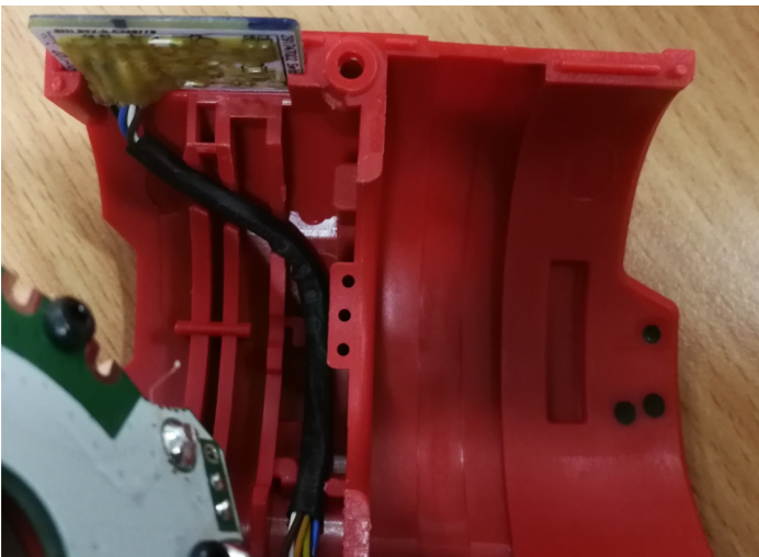
STEP 5: Install the pop switch into housing half as shown. Route wires through traps being sure wires are tucked completely down.
