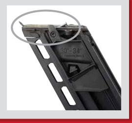
**STEP 4:** Use tool to remove jammed nail.
