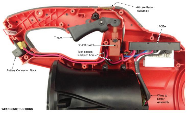
As an aid to reassembly, take notice of wire routing and position in wire guides and traps while dismantling tool. Be careful and avoid pinching wires between handle halves when assembling.
