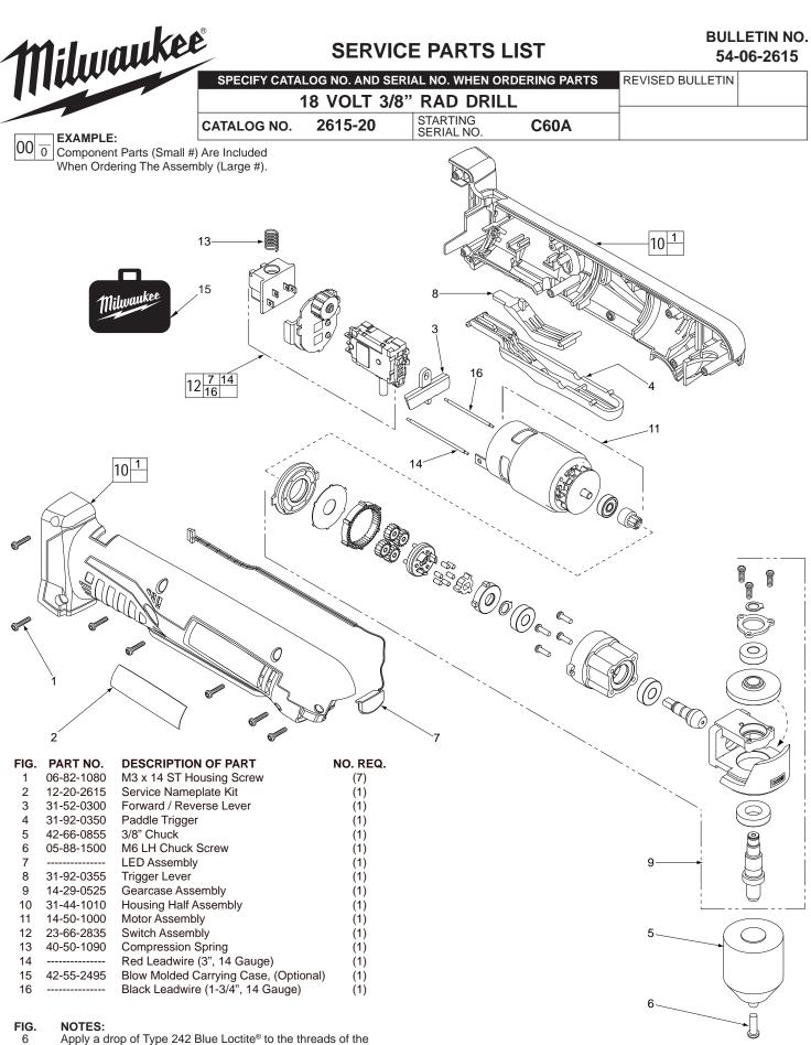
chuck screw (6) before securing chuck (5) to the spindle .
