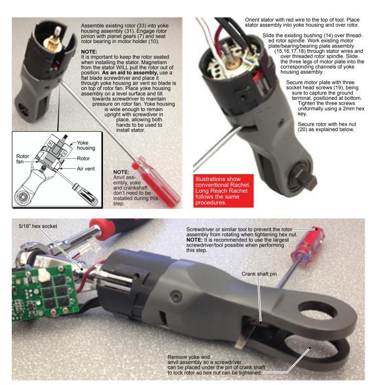
To properly tighten hex nut (20) to rotor (33), it is important to lock rotor and keep it from spinning. The recommended approach is illustrated above.
