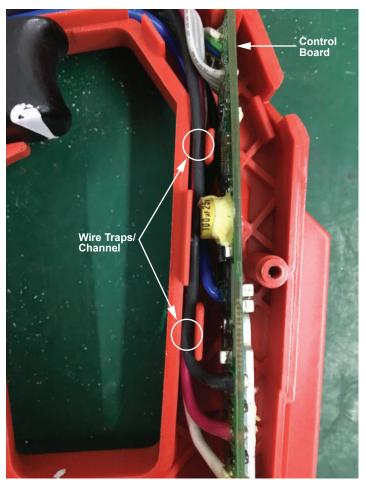
Route all control board wires through wire traps/channel as shown. Be sure to push wires completely down in traps. Be sure control board is seated squarely and firmly in support housing.
