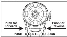
For **forward** (clockwise) rotation, push the control switch in the direction shown. Check the direction of rotation before use.
