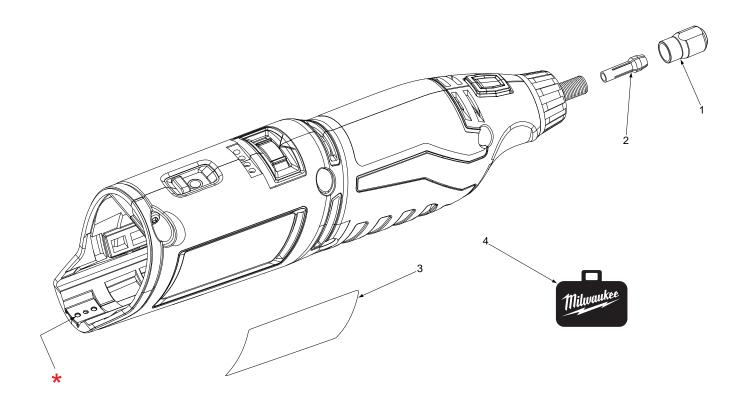
42-70-0058 \* 0 Improved Design 0 Original 0 Design 42-70-0055 0 M12<sup>™</sup> tools utilize two different Housing Connection Clip designs depending on the Handle Set . See page two for details.
