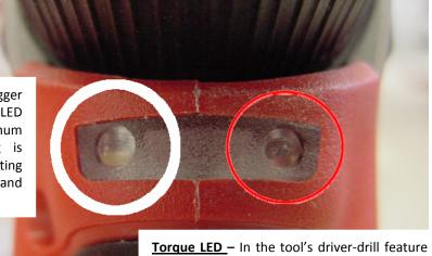
with Trigger pulled - the Torque RED LED Light doesn't illuminate until the maximum torque output for the clutch setting is reached; the tool will stop and the RED Torque LED will flash / blink approximately 6 times and then 'go out'... release the switch to reset.
