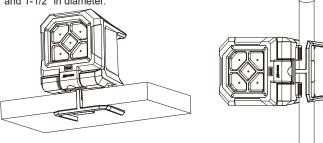
**Rotating the Face** To rotate the face, tilt the face forward and rotate up to 150° one way,
