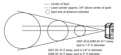
2267-20: At 5' away, spot is 6" in diameter 2268-20: At 5' away, spot is 5" in diameter
