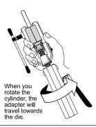
5) Begin squeezing the lever and continue until the edge of the adapter meets the die or pumping action shows substantial resistance.
