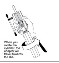
Begin squeezing the lever and continue until the edge of the adapter meets the die or pumping action shows substantial resistance.
