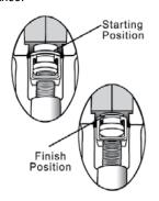
7) Grasp the yoke and rotate the tool counter-clockwise to remove the adapter from the die
